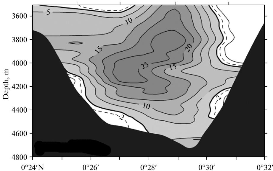
Fig. 3. Component of the currents normal to the section in the Romanche Fracture Zone measured using the LADCP instrument in November 2009.
