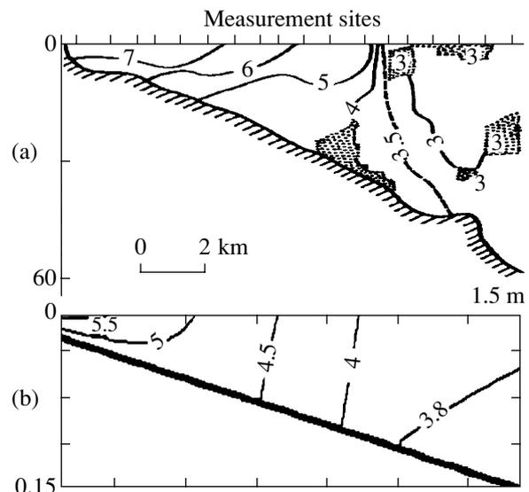
**Fig. 2.** Cross-sectional distribution of water temperature (a) in the southern part of Ontario Lake during the period of existence of a thermal bar (according to [5]) and (b) in the laboratory basin.
