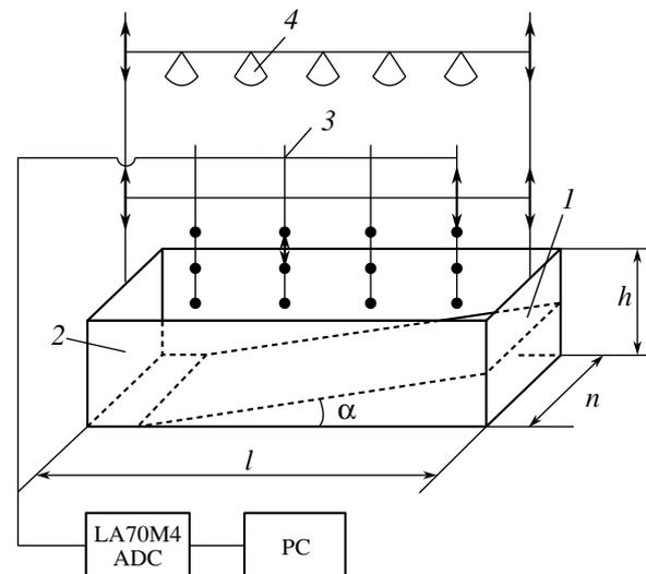
**Fig. 1.** Schematic of the laboratory setup:  $l$  basin length,  $\alpha$  bottom tilt,  $n$  basin width,  $h$  basin depth,  $l$  inclined bottom (wedge), 2 transparent observation window, 3 vertical probes with thermal sensors, and 4 electric bulbs.
